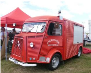
One particularly interesting vehicle was a 1967 Citroen model type H. Conceived as a delivery van, the H-van employed the characteristic Citroen front wheel drive to provide a very low loading height together with full standing. The distinctive corrugated panel work provided rigidity and permitted the use of thin-gauge steel sheet. Imported from France in August 2013 it is now a retired fire truck.
